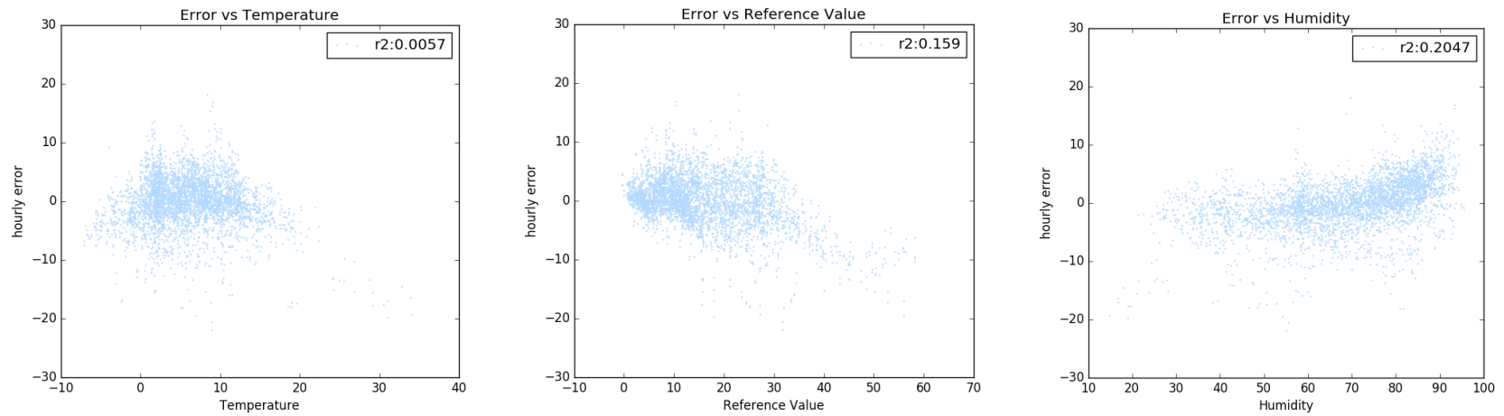
Figure 17. PM2.5 error across the range of ( left ) temperature, ( middle ) reference PM2.5 concentration values, and ( right ) relative humidity
